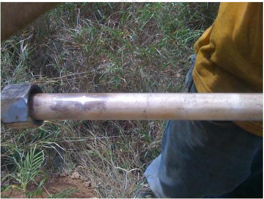
Photograph 2: Typical soil core collected using slide hammer within the PCB contaminated grid.
