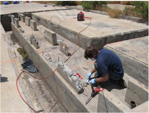
Photograph 10: Collecting dust samples from the concrete slab within DU-4. Direction: Facing West-Northwest.
